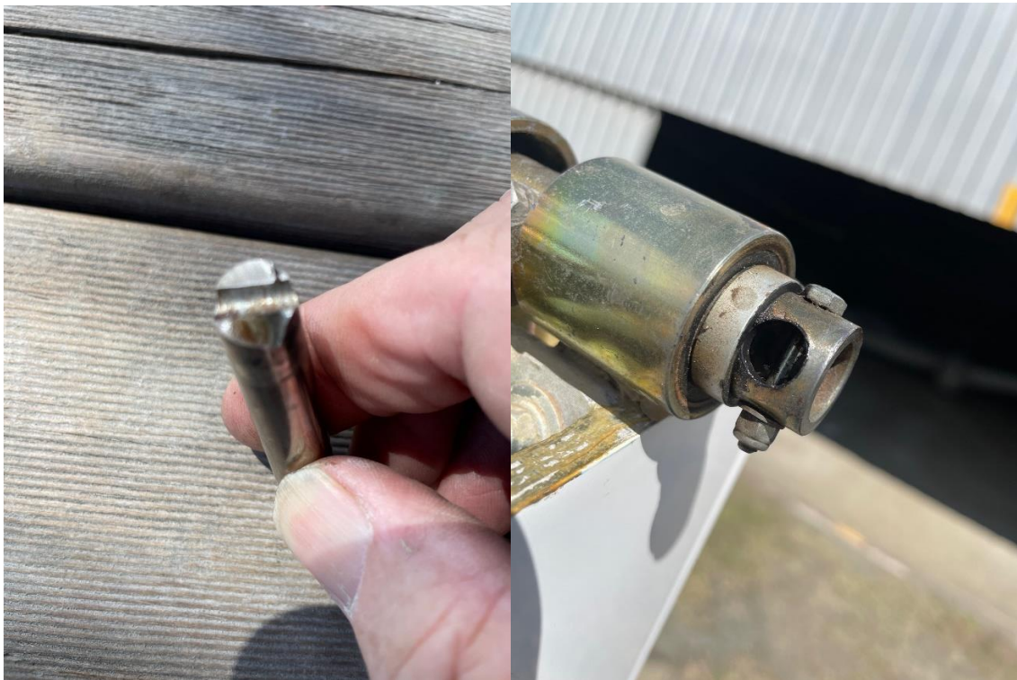
Figure 1: The affected sailplane on the daily inspection showed excessive tailplane lateral play. The pin fracture occurred at the attachment bolt.
