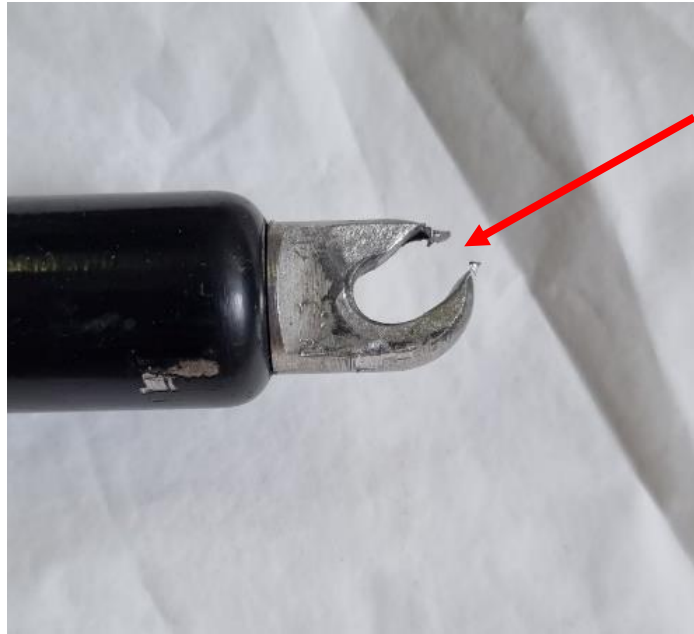
Figure 2: Close up of torn fitting.
