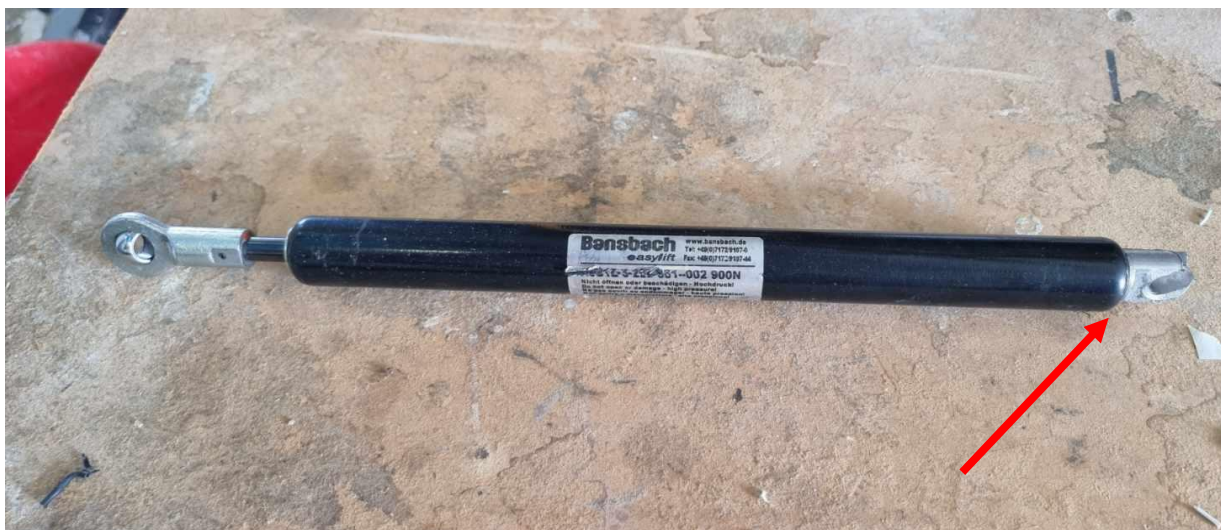
Figure 1: DG 800 gas strut attachment assembly with torn fitting.
