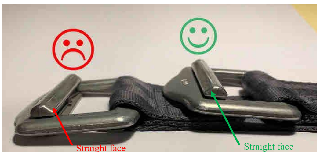
Figure 1: Left adjuster is wrong; straight face of slider is towards webbing. Right adjuster is correct; straight face of slider is towards adjuster nose.
