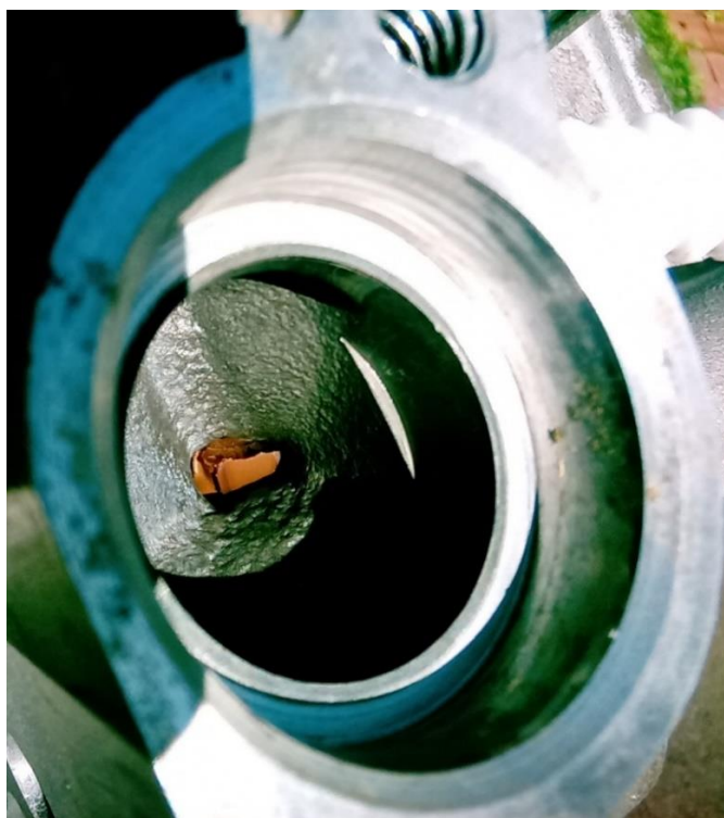
Figure 1: Blockage of cylinder head coolant port.
