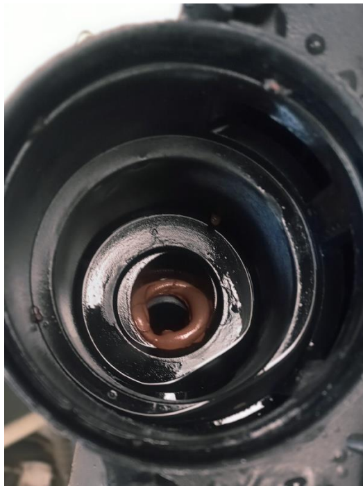
Figure 4: Excess sealant / adhesive squeezed out into inside of heat exchanger.
