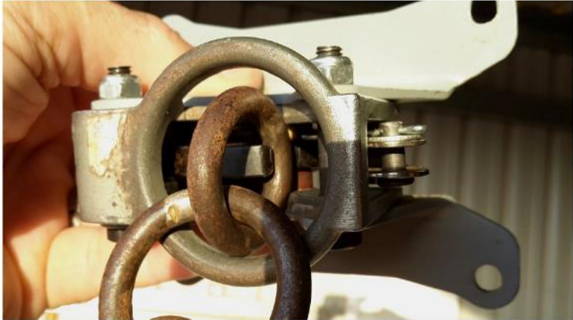
Figure 2: TOST E 22 release. Worn rings wedging under beak.
