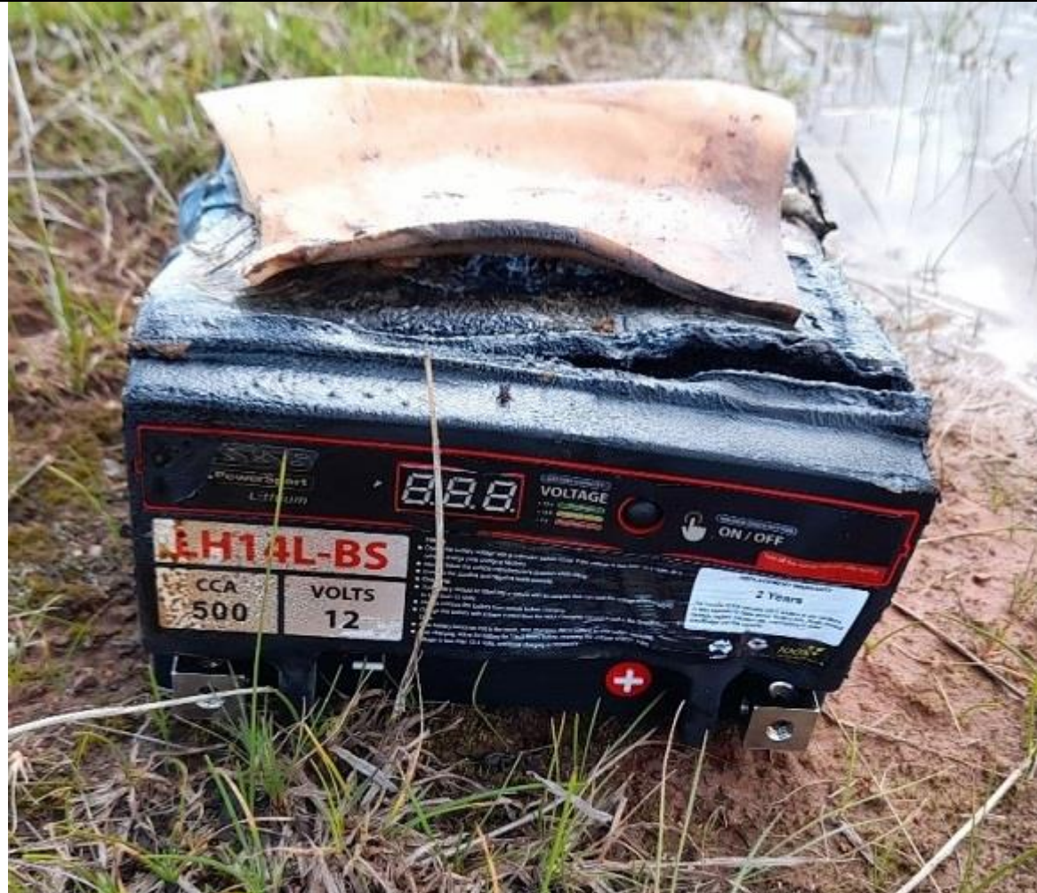
Picture: Smouldering battery after removal from aircraft.
