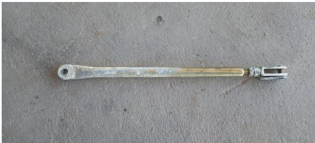
Figure 1: Corroded rear release pushrod resulting from water and urine exposure.
