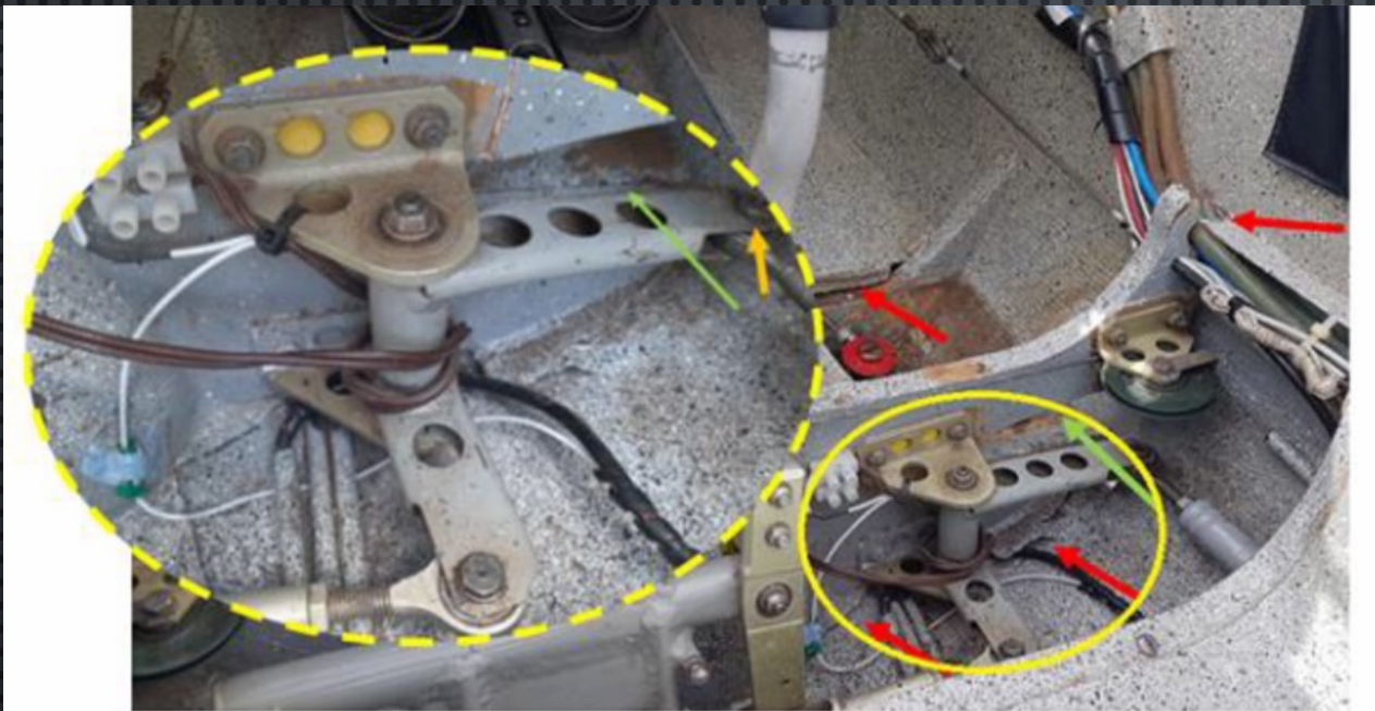
Photo 4 - The nut on the bolt (orange arrow) contacted with the bulkhead preventing movement of the bell crack through the cavity (green arrow).
