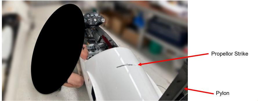
Recreation of engine operator position post incident. Sailplane has been moved into a workshop. Propellor strike on upper fuselage. Propellor pylon visible at bottom right.
