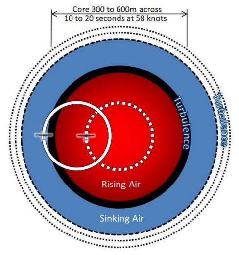
It is important to develop a <u>mental picture</u> of the rising air and the location of the core by feeling the surges and monitoring the instruments. Centring is the process of moving the circle a little in the direction of the core – no more than one adjustment per complete circle.
