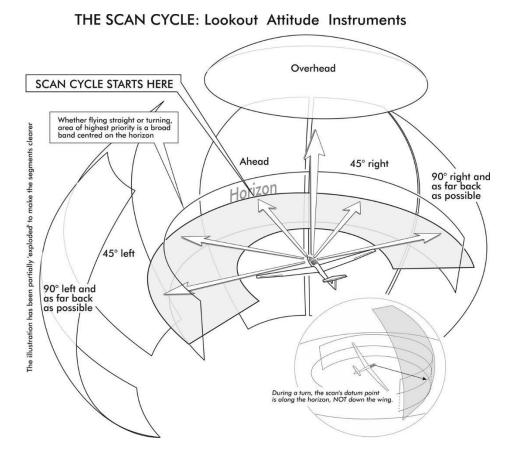
We may also have aircraft coming from the side, across out flight path, or overtaking us on either side, so we also need to monitor these areas. The technique is to focusing on a spot for a few seconds, then moving our view 20-30 degrees ahead and repeating the process.
