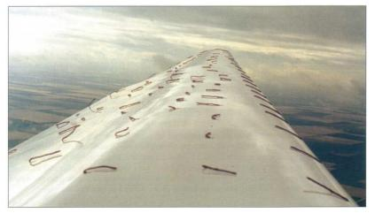
The airflow in this picture (flowing over the wing from right to left) is shown by wool strips taped to the glider wing.
