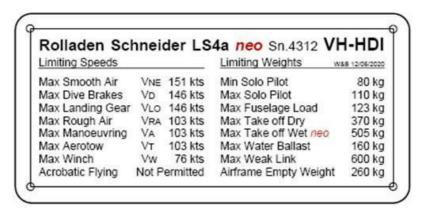
The permitted aerobatic manoeuvres will also be displayed, either on the same placard or on a separate one alongside. The maximum (and possibly the minimum) weak link strength will be displayed, internally on the placard and externally next to the release hook(s).
