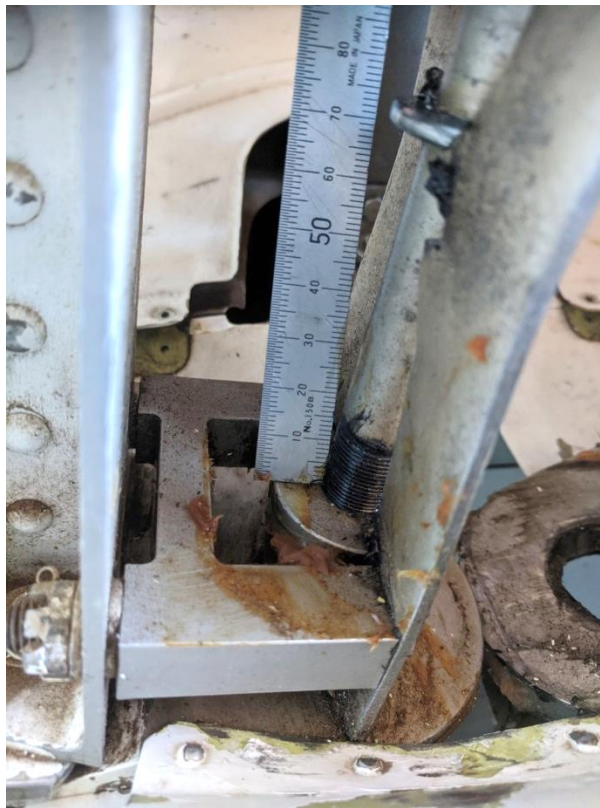
Incorrect rigging - 13 mm thread exposed, collar not retained in slots, wear / contact surfaces visible on tapered bolt. Centre collar is above slot in guide plates
