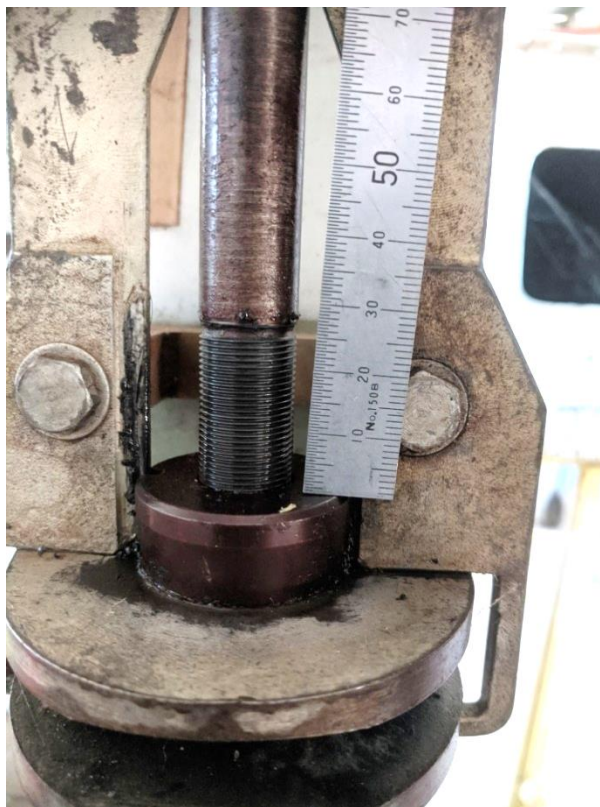
Correct rigging - aligned spar fittings and 25 mm thread, no wear / contact surfaces on tapered bolt exposed, collar housed in retainer.
