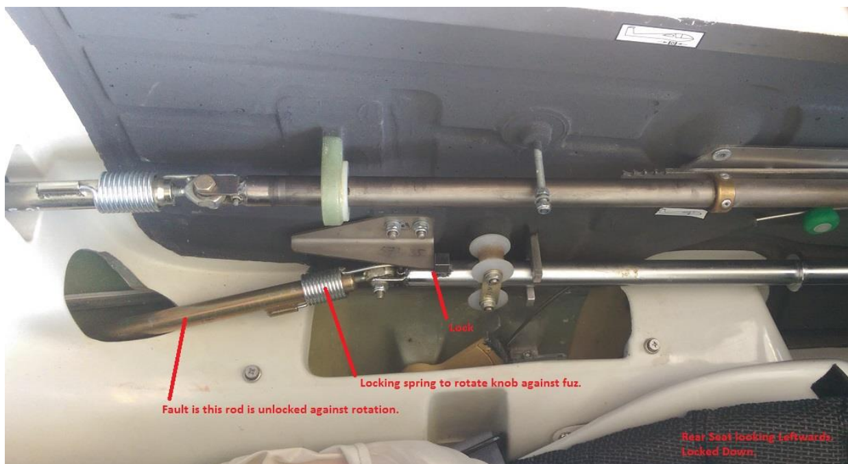
Figure 1: Undercarriage push rod in left rear cockpit
