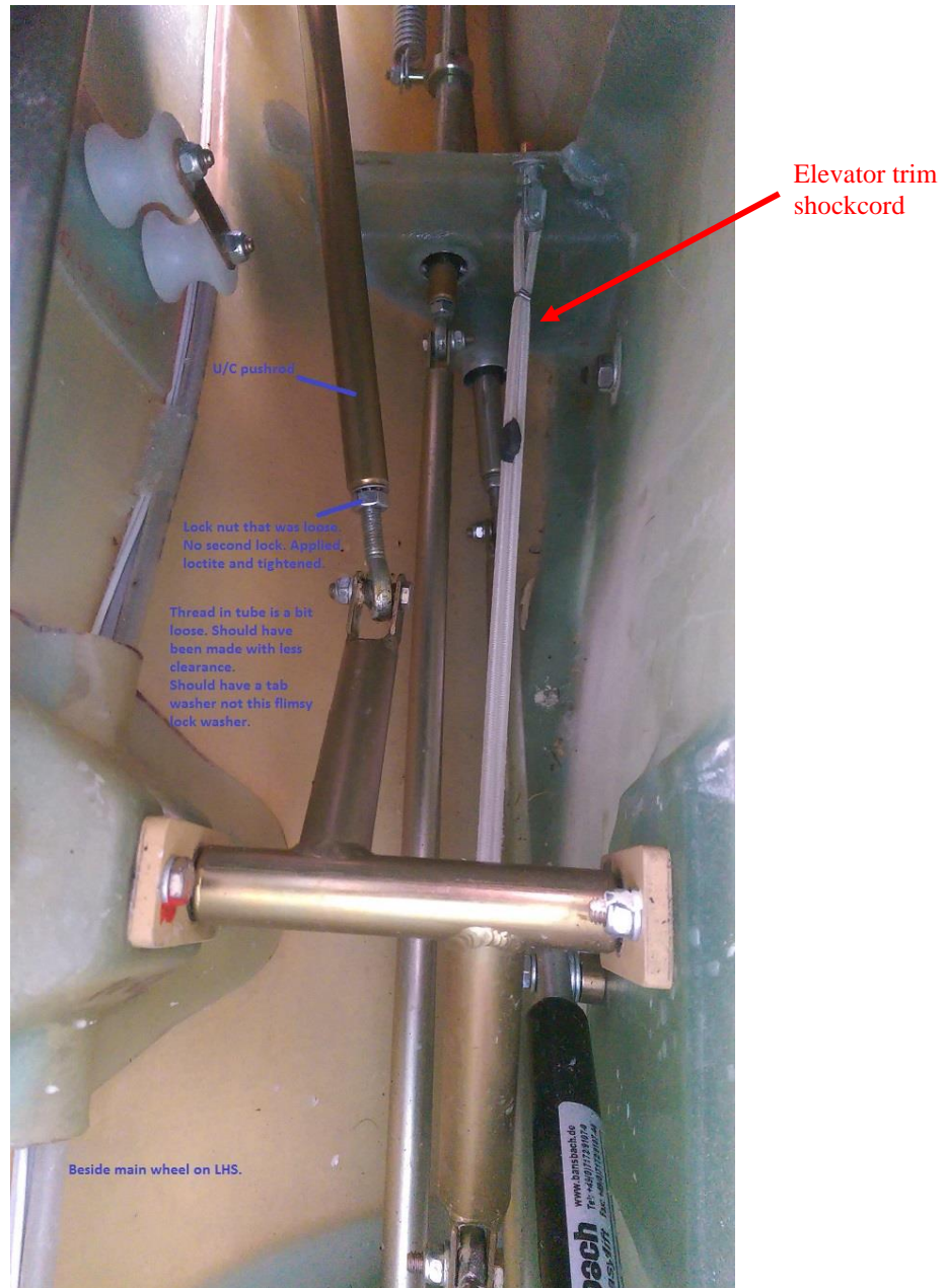
Figure 2: Undercarriage push rod in centre fuselage. Elevator trim shockcords are on right hand side
