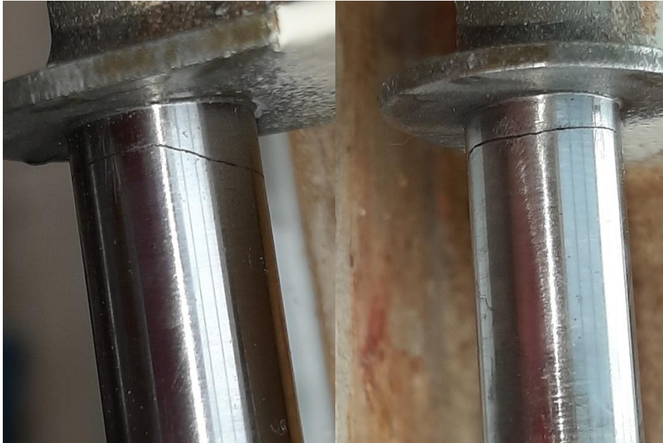
Circumferential cracking of the chrome plating near base of spigot
