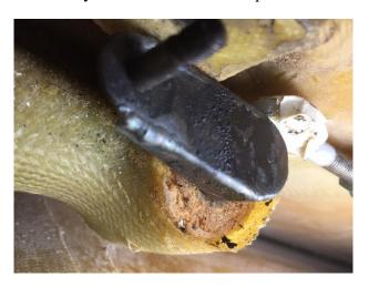
NEWLY RE-WELDED ACTUATOR ARM INSIDE THE WING
