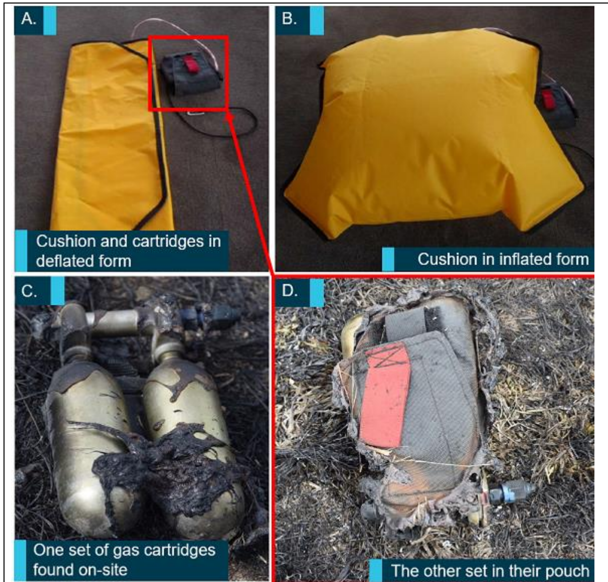
Figure 9: The components of the egress assist cushion. Source: ATSB
