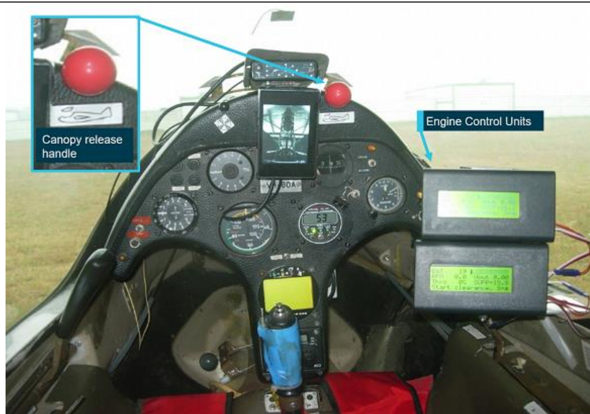
Figure 5: View from front seat in GOA's cockpit. Source: Flight Manual, amended by the ATSB
