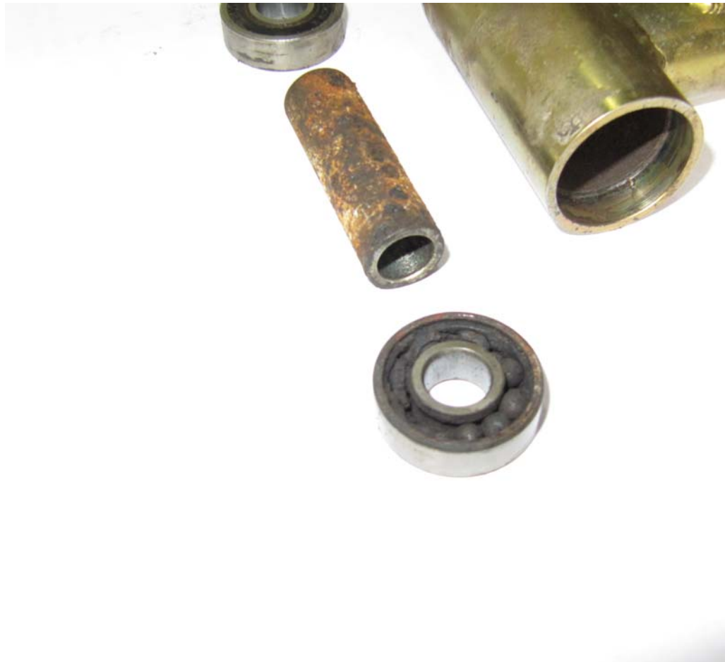
Damaged Dive Brake Pivot Arm Bearing and Corroded Spacer Tube Removed from DG 500 Glider VH-VMF
