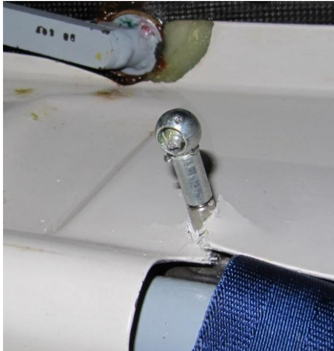
Figure 2: Gas strut end protruding through parcel shelf.
