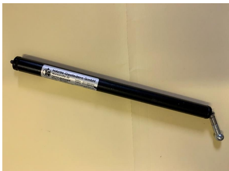
Figure 3: Failed gas with bent strut.
