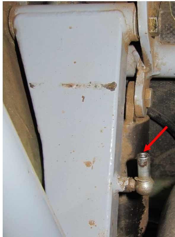
Figure 1: View in the wheel wheel looking forward showing port undercarriage arm and disconnected gas strut connection
