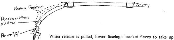
when release is pulled, lower fuselage bracket flexes to take up slack in guide tube/adjuster. This decreases the travel of the inner cable, which then does not provide full travel to the release hook, as well as making adjustment impossible.
