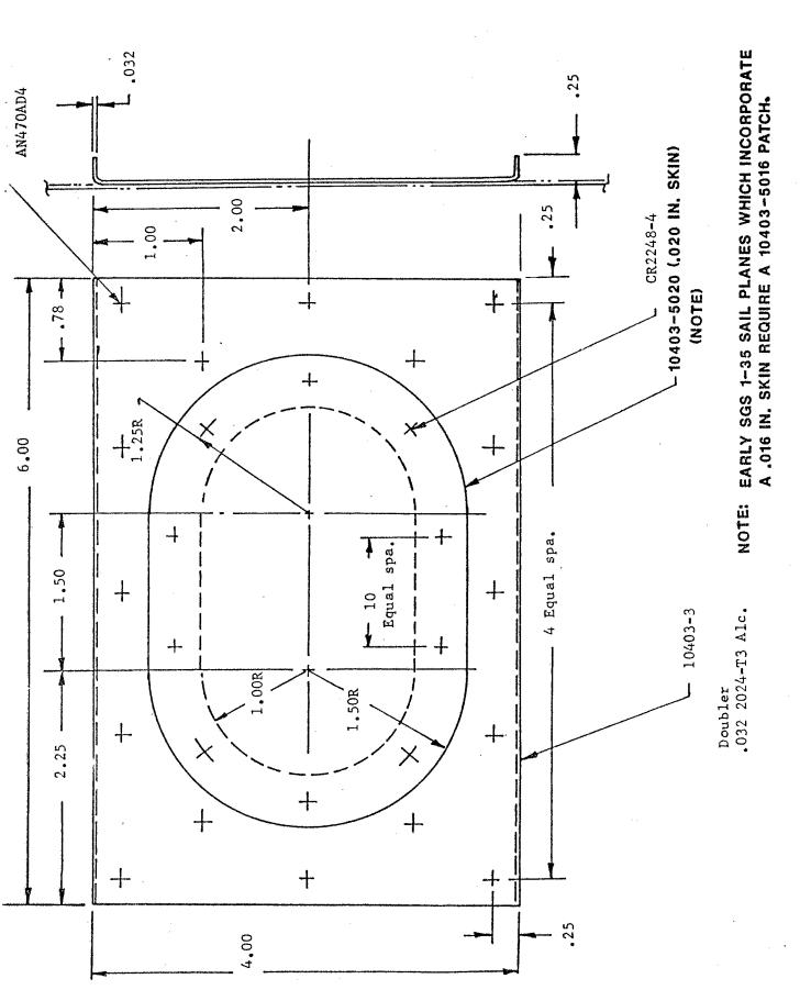
FIGURE 5. STRUCTURAL DOUBLER ID PATCH
