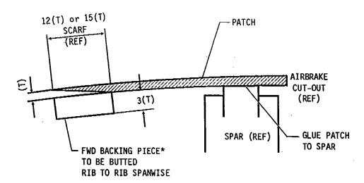
\*FORE AND AFT BACKING PIECE TO BE BUTTED BETWEEN FWD BACKING PIECE TO SPAR
