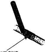
If any suspicions exist, use a penetrant dye. If a crack is detected to one of the two control handles, stop the glider from flight and order new handles to IAR – Braşov.
