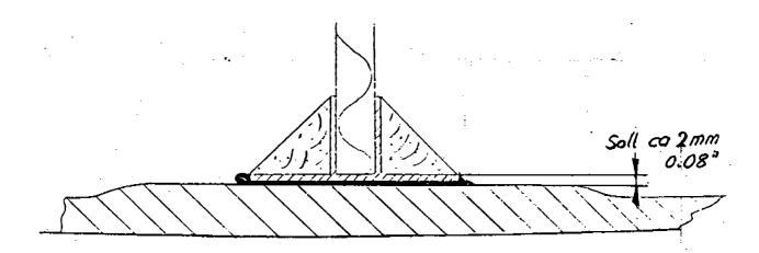
3.2 Overthick bonded joints may well include entrapped air bubbles, if the resin had not been properly squeezed out. Receding glue line must be viewed with suspicion. In both these cases a repair according to Appendix II must be carried out. The extent of the fault will be determined by means of probe drillings. Probe drillings shall be carried out within the suspected area, starting from inboard, in accordance with para. 4.
