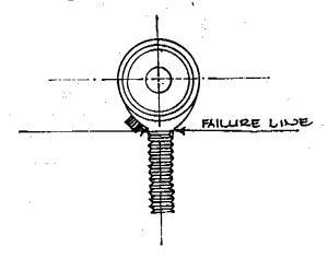
Should your aircraft be subject to a heavy landing this area must be checked thoroughly for evidence of failure.
