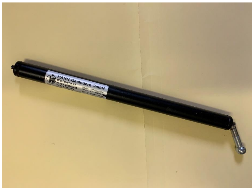
Figure 3: Failed gas with bent strut.
