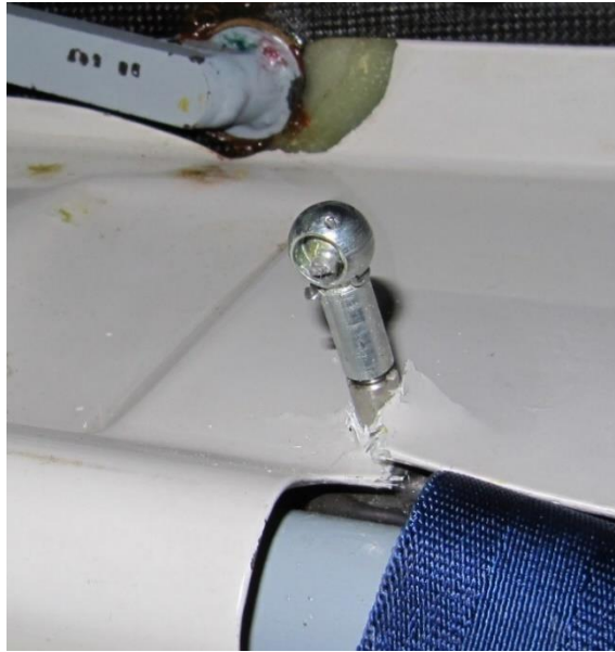
Figure 2: Gas strut end protruding through parcel shelf.
