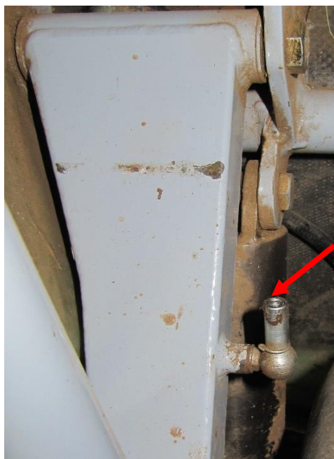
Figure 1: View in the wheel well looking forward showing port undercarriage arm and disconnected gas strut connection
