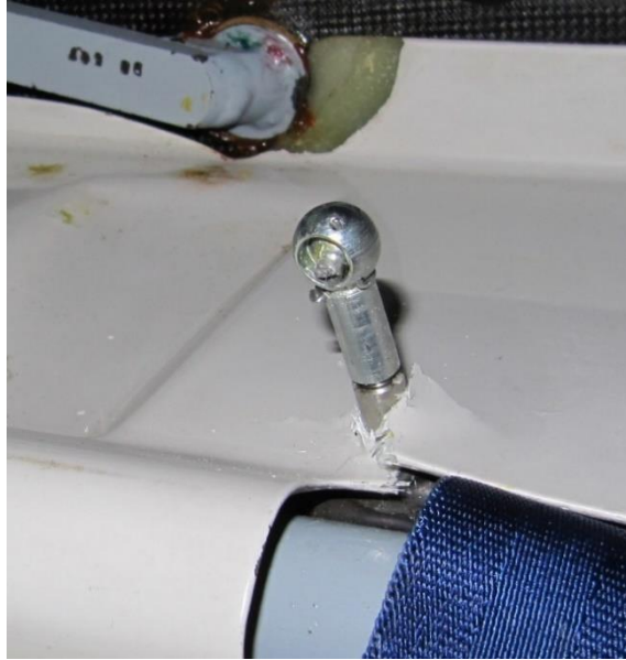
Figure 2: Gas strut end protruding through parcel shelf.
