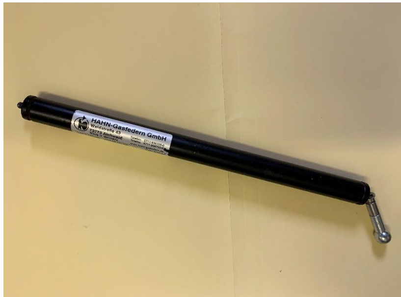
Figure 3: Failed gas with bent strut.
