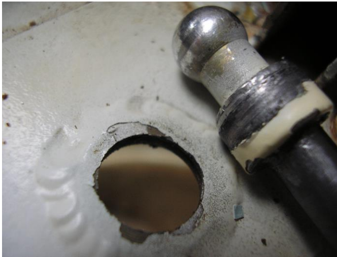
Photo 2. Left hinge pin failure area.
