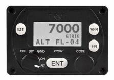
ADS-B (Automatic dependent surveillance–broadcast) – New portable low-cost transceiver equipment has recently been approved by CASA. Air Traffic Control, TCAS equipped aircraft and Flightradar24 can track the glider so equipped.
