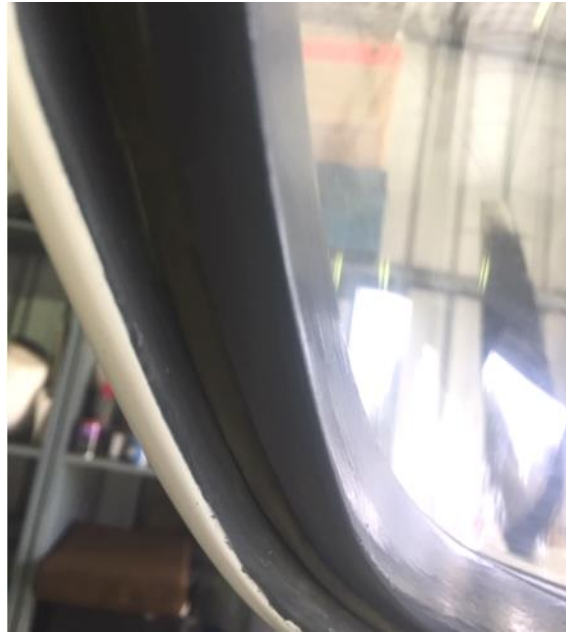
Figure 7: Canopy Seal In Good Serviceable Condition.
