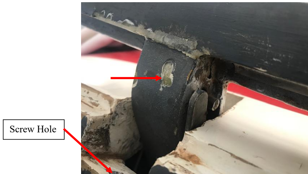
Figure 10: Example of Screw Head Interference With Canopy Hinge
