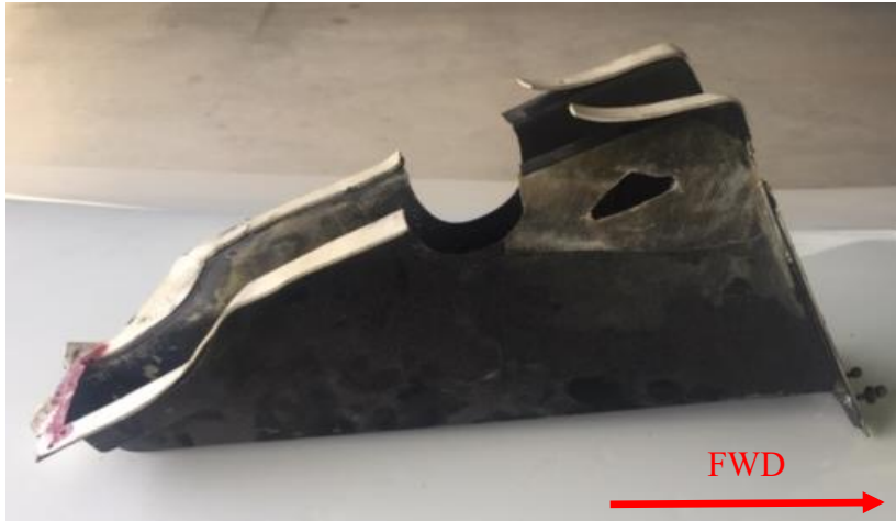
Figure 8: Canopy Strut Cover Removed from Aircraft.
