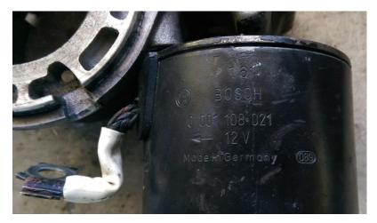
The same starter configuration is used on some Limbach L1700, L200, and L2400 engine versions, not all. The LMS574 could be used on the similar installations as per this EO. This should suit all Limbach engines with the adjacent Bosch serial number, 0 001 108 021, starter whether it was modified by Limbach or not.
