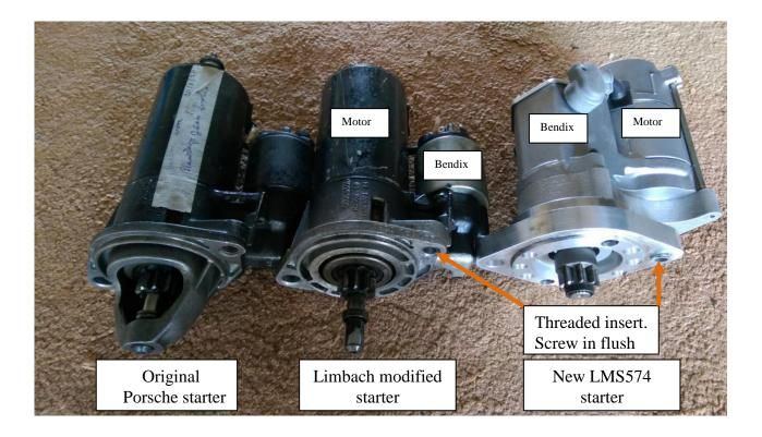
The original Bosch starter motors were made for a Porsche 944. They were modified by Limbach to suit by trimming the nose, as shown. This nose bearing is provided by the Limbach in the accessory case. It also has an insert in the one mounting hole. The shape of the alternative starter motor is different but similar. The cable attachment points and size are similar enough to fit without changes, except as noted in the EO.
