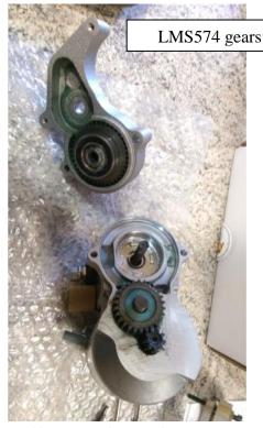
The LMS574 appears to be a more robust modern construction and has a good reputation as a robust well made starter. It is also intended for the Porsche 944 car and required only minor modifications to suit. In fact less modification than the original starter as discussed below.
