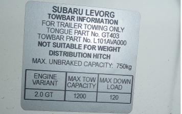
Recently GFA received a report of a Tow Bar falling of a vehicle while the glider trailer was attached. Fortunately the driver suspected that something was not quite right and stopped to check. Some manufactures stipulate in their vehicle operating and service manuals that
