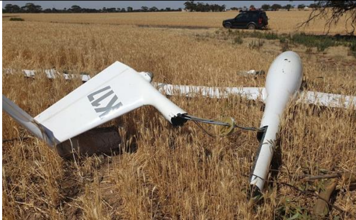
Figure 4: Tail Displacement Showing Intact Control Runs
