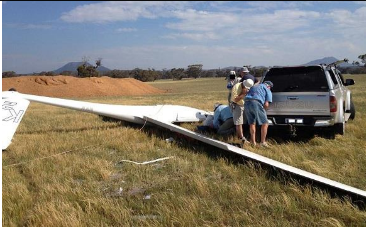
Fig 2. Wreckage showing impact point in the foreground identified by broken canopy fragments.
