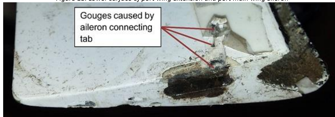
Figure 19: Close up of gouging on lower surface of port main wing aileron.
