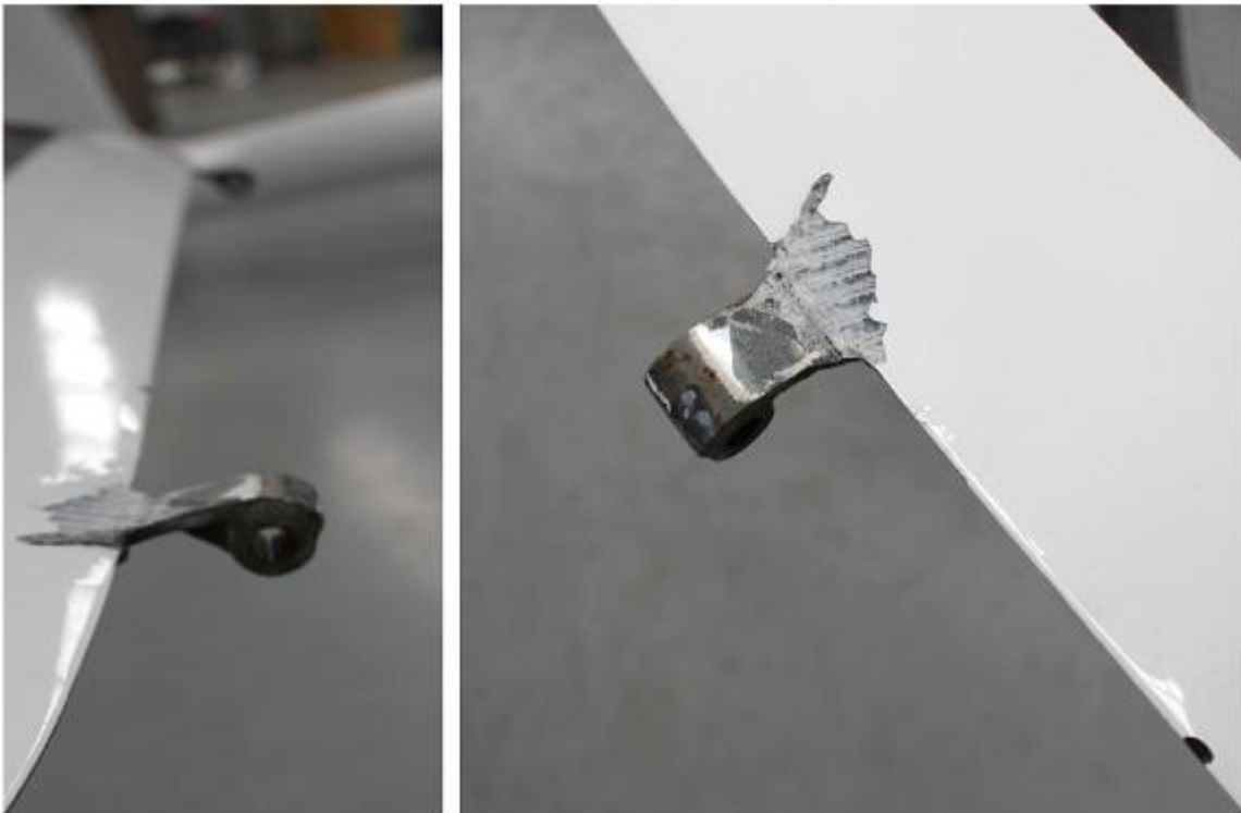
Figure 3. Hinge over-extension and supporting structure damage
