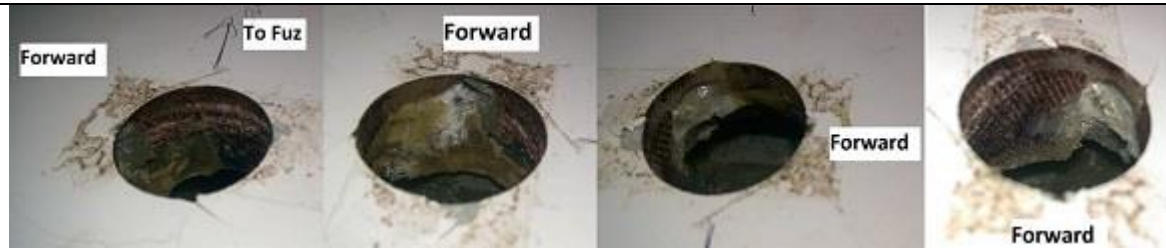
Figure 13: Retaining pin hole location in wing (each photo rotated 90 degrees).
