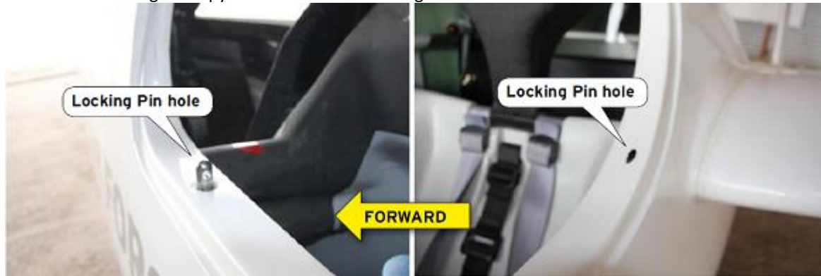
Figure 9. Mating location of the locking pins on the fuselage
