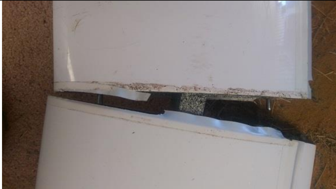
Figure 11: Wing extension Demonstrating Failure Method.
