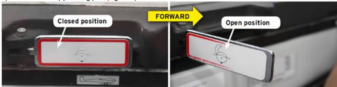
Figure 7. Closed and open positions of canopy locking handle
