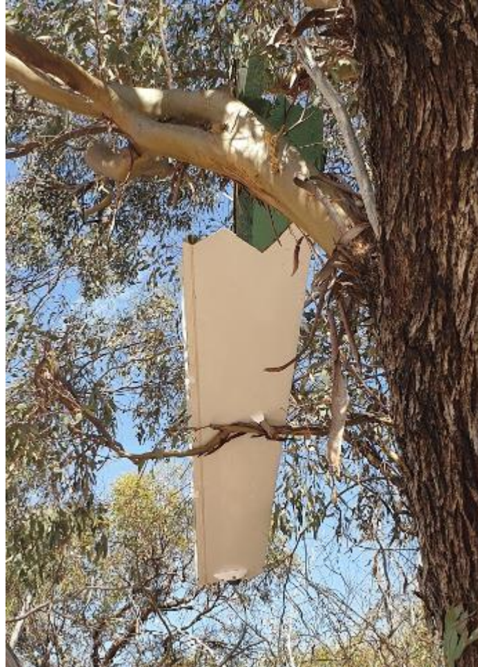
Figure 6: Port Main wing Impact with Tree
