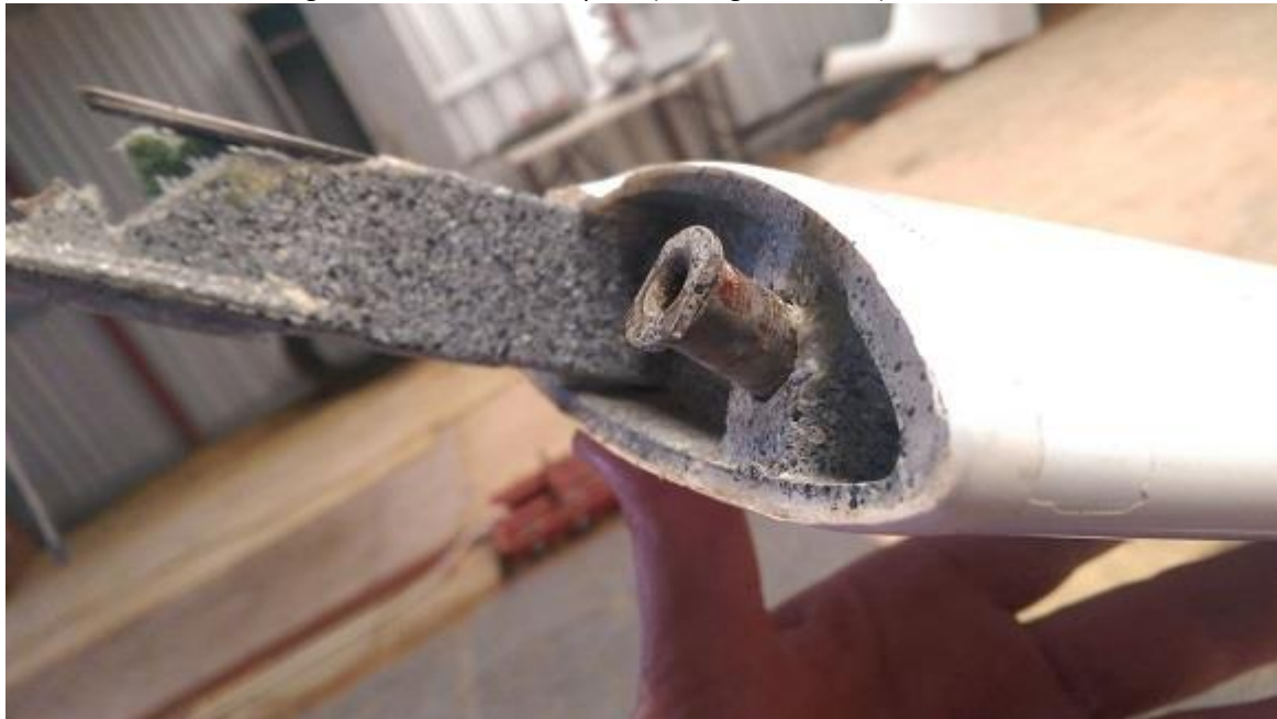
Figure 9: Extension Forward Shear Pin Bush, reinserted In wing extension, demonstrating the sequence of failure.
