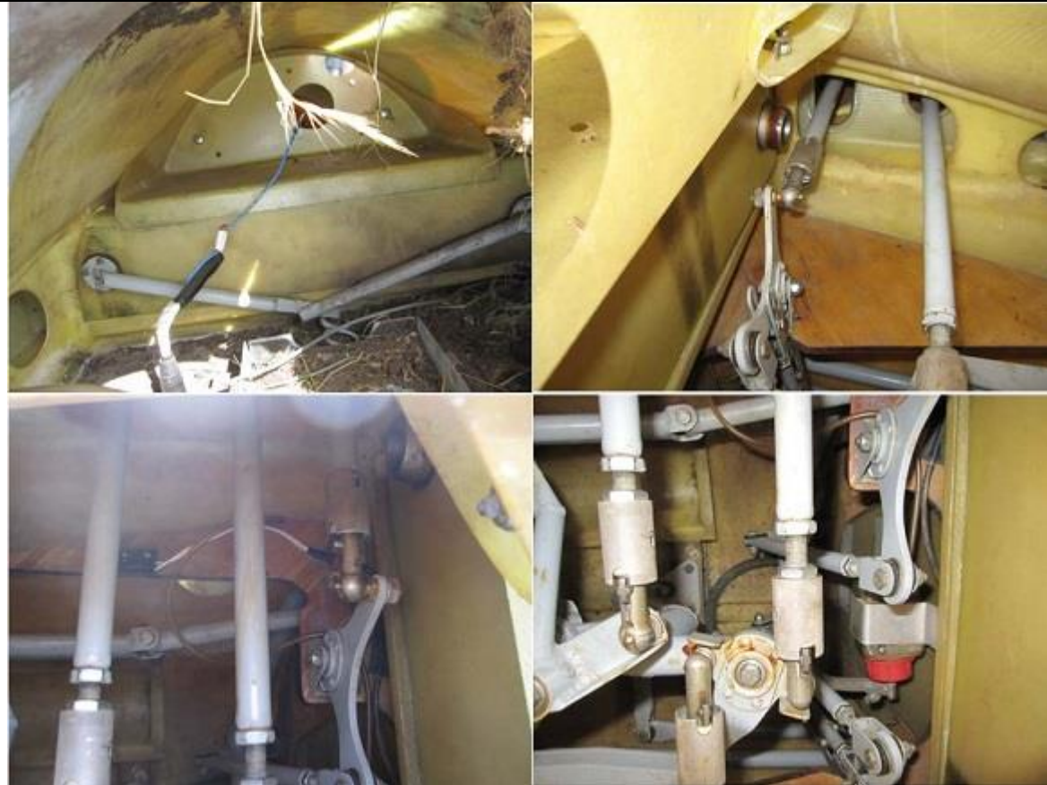
Fig 5. Main pins and control linkages intact.
