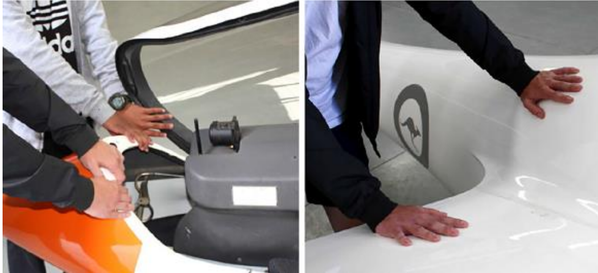
Figure 11. Pulling from nose and pushing via the wing root
