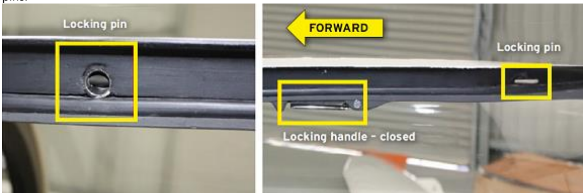
Figure 8. Rear canopy locking pin(s)
