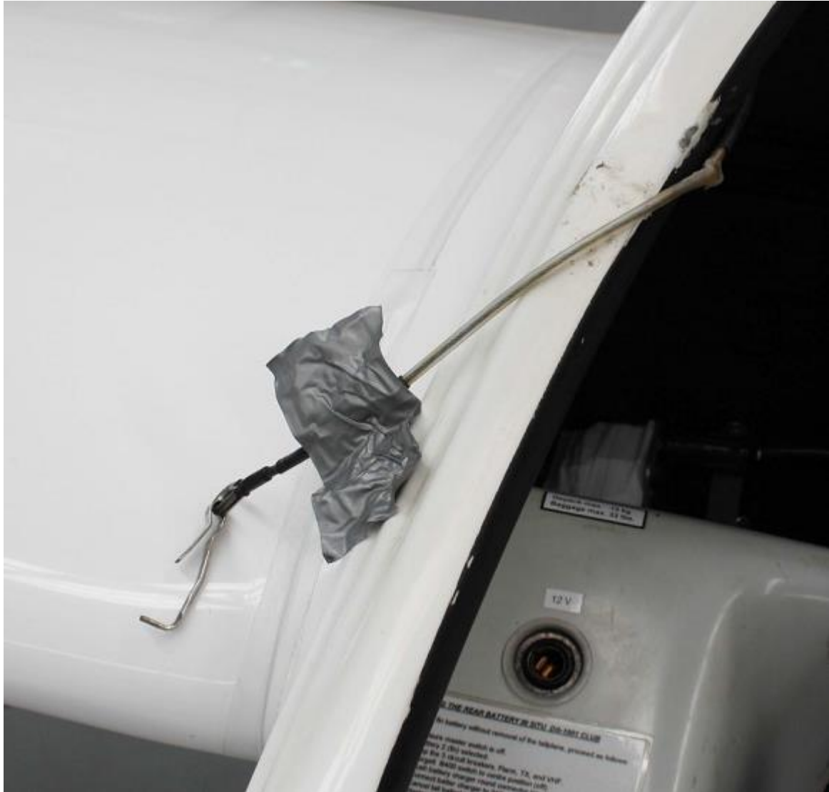
Figure 4. Retaining clip over-extension damage
