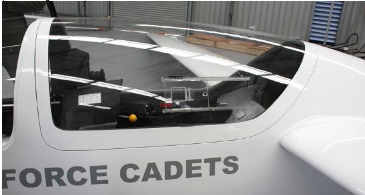
Figure 10. Rear canopy flush with Fuselage
