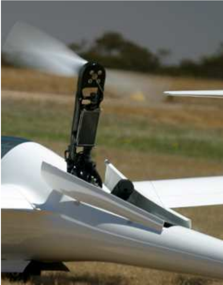
Figure 33-4 The arresting wire and engine doors can be seen.
