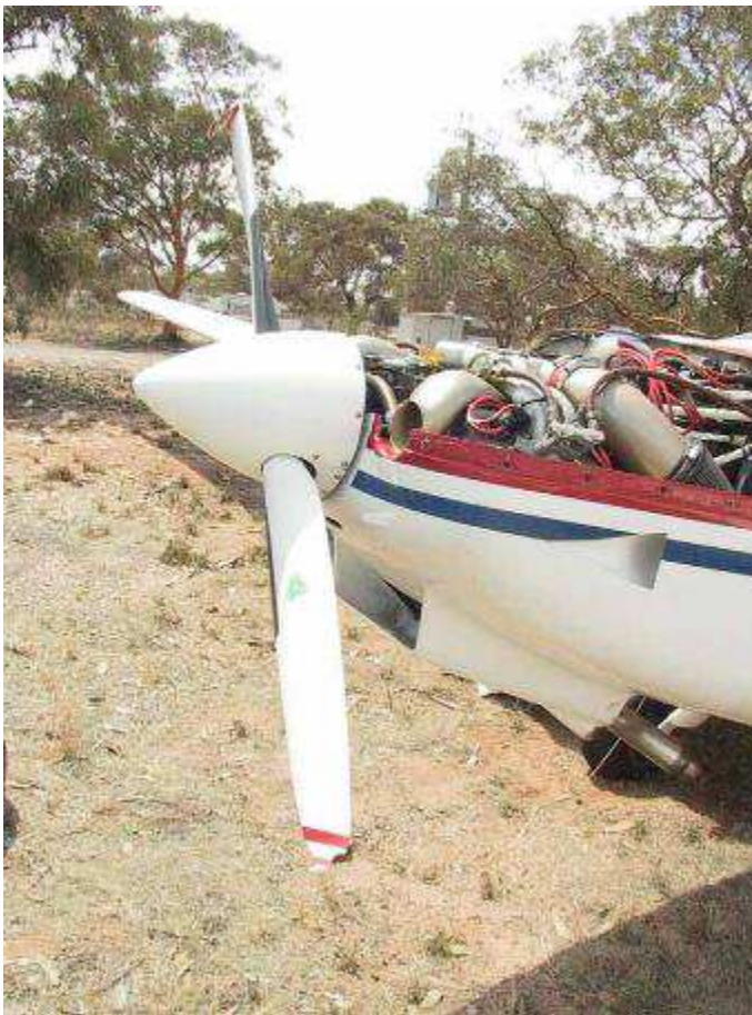
Figure 26-1 G109 with Limbach L2400DFI 100HP and MT Electric Propeller.
