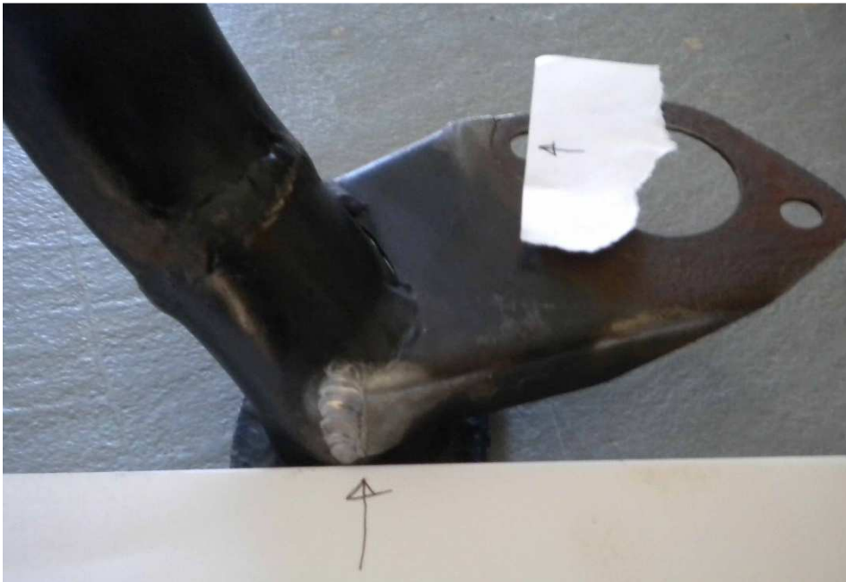
Figure 31-2 Intake Manifold for a Limbach L2000EB1AC Cracked at a weld and in the material where it mounts on the Cylinder Head.
