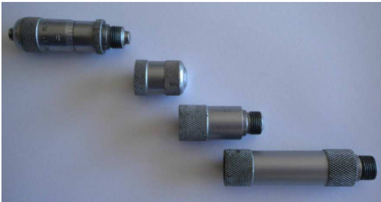
Good quality internal Micrometer
