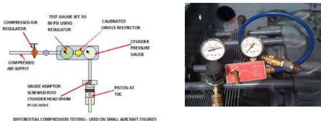
Figure 9-7 Differential Pressure Testing
