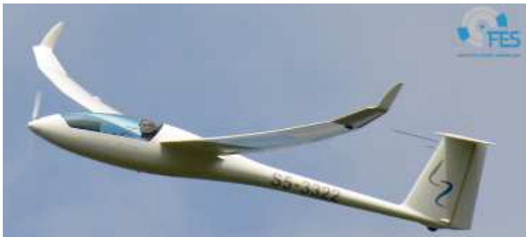
Figure 12-1 Ventus 2Cxa with FES motor and rear folding propeller
