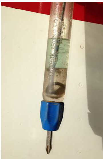
Figure 14-1 Water found in a Pawnee tug after it had stood out overnight in rain.
