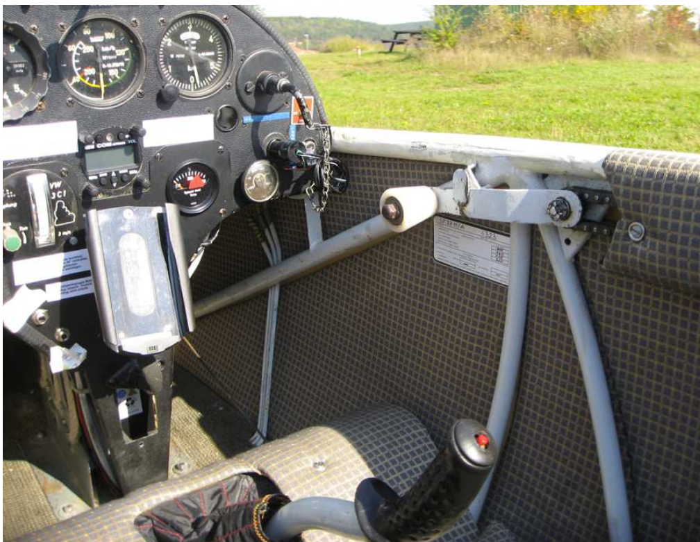
Figure 33-2 Chain drive of the SF27M connected to the mechanical handle
