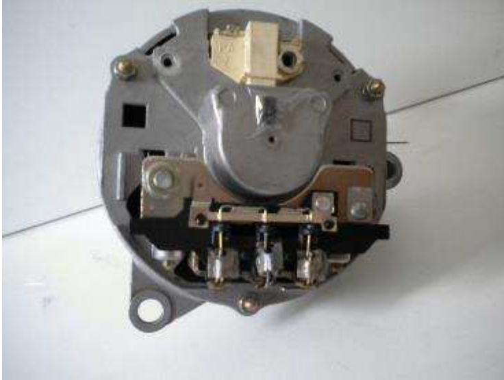
Figure 21-2 L2000EB1A alternator with rectifier diodes showing
