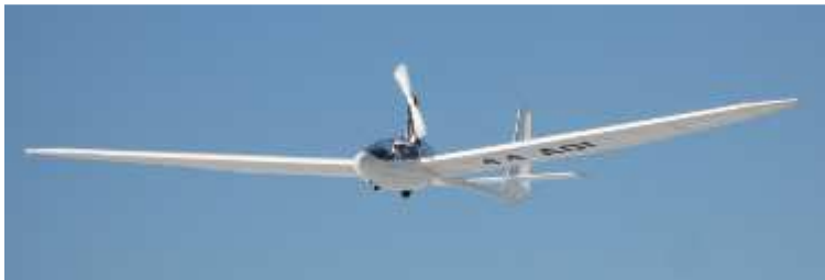
Figure 12-2 Alatus ME. With Electravia electric propulsion system
