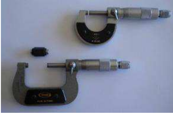
Above a 0-25mm and a 25mm-50mm Micrometer. Note the checking staff for the 25-50mm Micrometer
