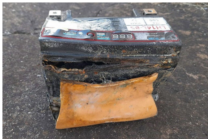
Figure 18-1: LFP Battery Used As A Starter Motor Battery That Was Overcharged Inflight
