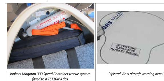
The rocket-deployed emergency recovery parachute systems are often cable activated by the pilot via a red handle.
