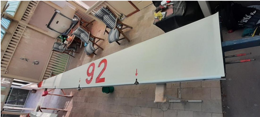
Figure 3: Inverted Stbd Wing Showing Location of Cracked Spigots
