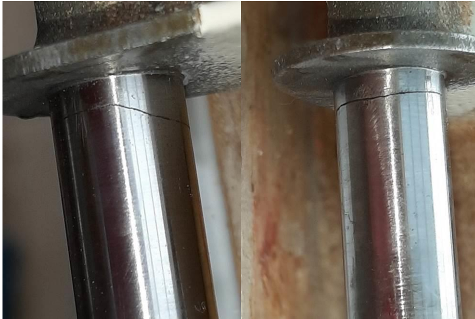
Figure 5: Circumferential Cracking Of The Chrome Plating Near Base Of Spigot
