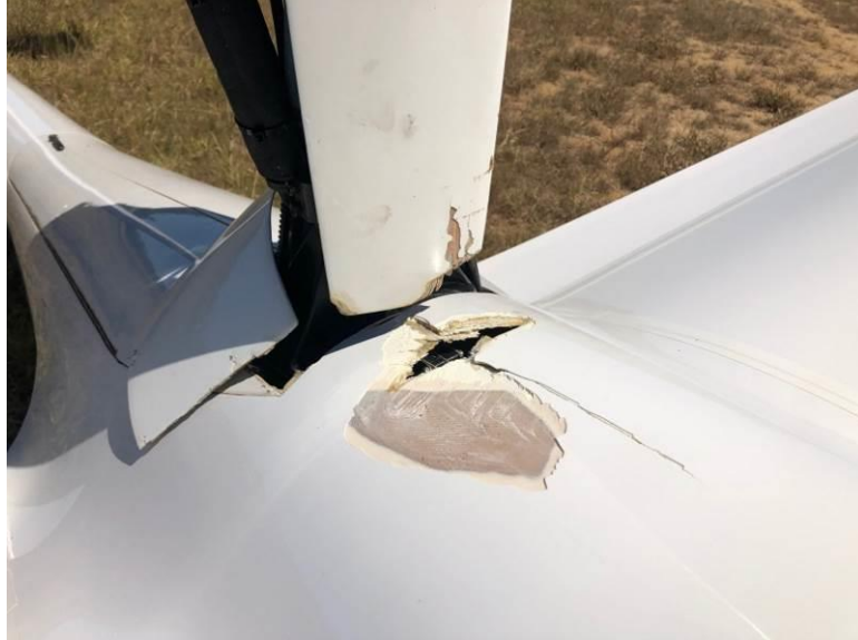
Figure 7: Damage to Upper Fuselage After Prop Strike From Broken Thrust Cable
