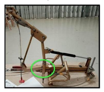
Repair welding work requires the four floor mounting points to be jigged to ensure the geometry is maintained and the part fits back in place. The repair should be carried out in accordance with an engineering order or approved data equivalent.
